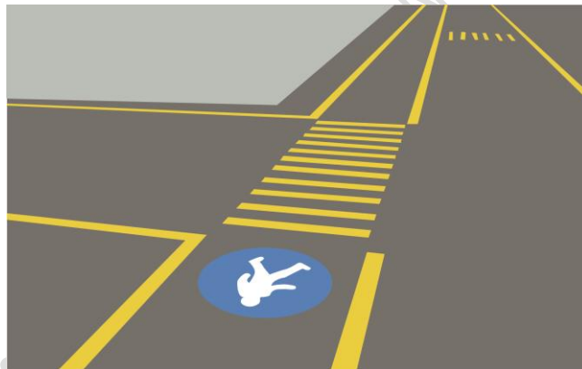
Fig. 5.3 – Yellow Demarcation for Pedestrian Pathway
